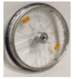
Rear wheel, drum brakes, 36 spokes, cross-wise spokes
